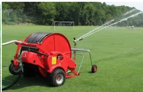
Figure 7: Travelling Sprinkler irrigation
