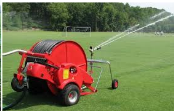
Figure 7: Travelling Sprinkler irrigation
