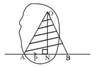
Suppose a force 'P' is acting along AB on a body. Body is free to rotate about a fixed point.
