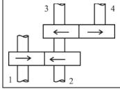
• At least one of the intermediate shaft have more than one gear in use.
